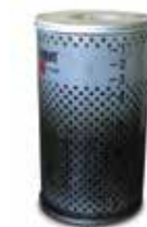
Fuel filter after 12,000 miles using typical #2 diesel.
